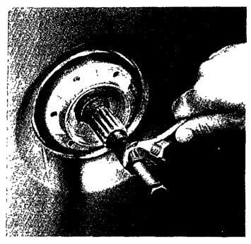
5 Turn the bolt against the center shaft to remove the lip seal from the center tube
